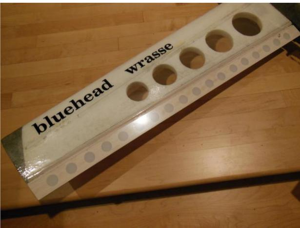
The wing comes shaped but needs to be sanded and stiffened with carbon rods top and bottom. It is covered with a material called "new stuff".
