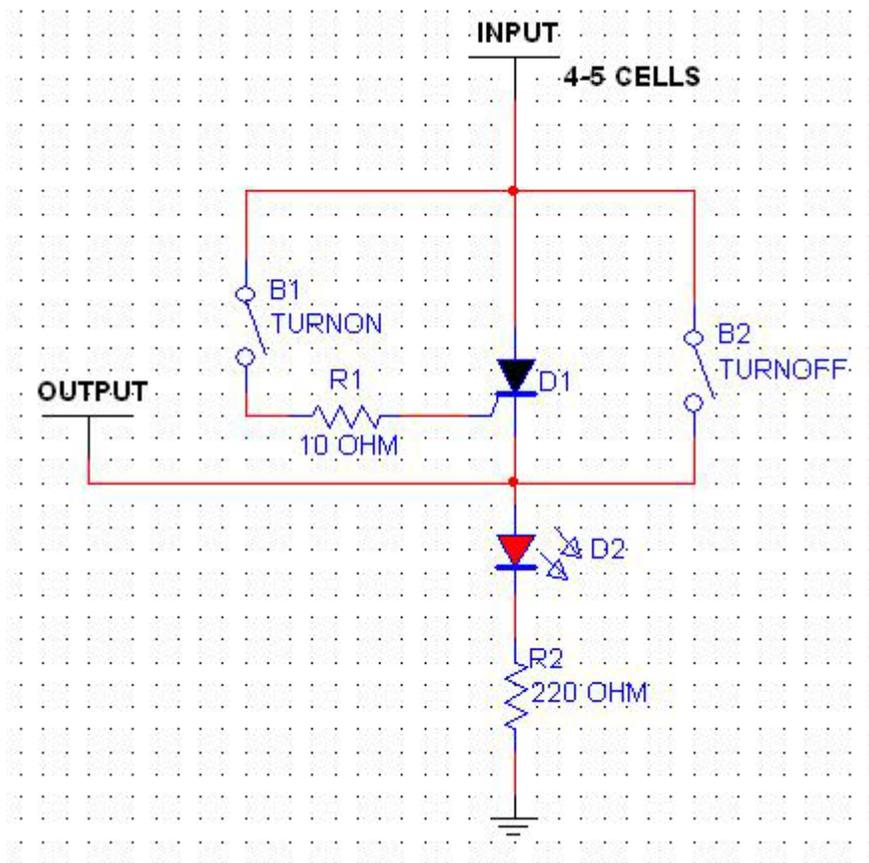
In the above schematic, your battery's positive input will be connected where the input is designated, and the negative of the battery will go to ground, represented at the bottom of the schematic. The output (positive switched voltage) to your receiver) is connected to the left, and the ground is again connected to the negative output lead.
